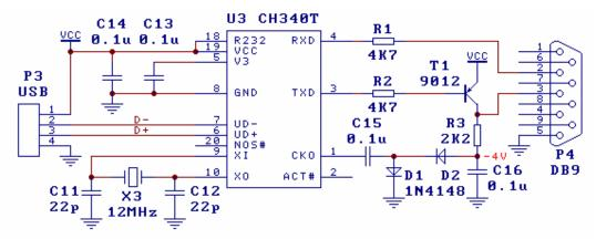
The image above is USB to RS232 converter design too, the function of this circuit is the same with 7.2 section except the range of output RS232 is narrower. When R232 pin is driven high, the assistant RS232 function will be enabled, just need to add some diodes, transistors, resistors and capacitors, the special level conversion chip U5 in section 7.2 could be replaced and the hardware cost is lower.
